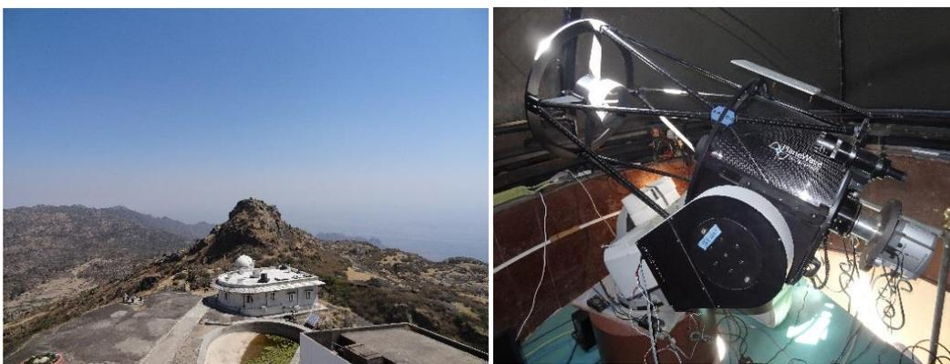
**Figure 2.1** - The dome and 50cm CDK reflector telescope
